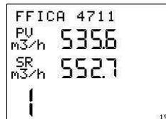
Fig. 3-7 Process value PV= flow A and SP = setpoint flow A
