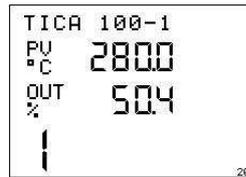
Fig. 3-21 Slave controller TICA 100-1 display, Controller output in display
