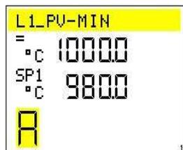
Fig. 3-3 Alarm value is set to 1000.0
